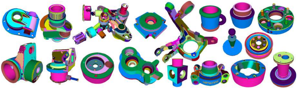
Fig. 9. Projection of the point cloud onto the detected primitives obtained from our segmentation algorithm. (For interpretation of the references to color in this figure, the reader is referred to the web version of this article.)
