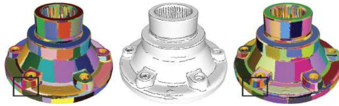
Fig. 4. Crest lines prevent the patches from spanning multiple primitives. Left: patches (without crest lines); Middle: detected crest lines shown in black (Yoshizawa et al., 2005); Right: patches from constrained region growing. (For interpretation of the references to color in this figure, the reader is referred to the web version of this article.)
