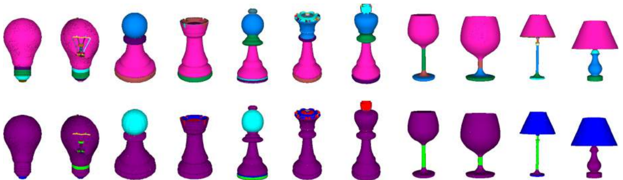
Fig. 13. Our segmentation algorithm for some models with surface of revolution. Top: Random colors for different parts. Bottom: Segmentation colored by primitive type (surface of revolution is purple, others are colored similar to Fig. 3H). (For interpretation of the references to color in this figure, the reader is referred to the web version of this article.)
