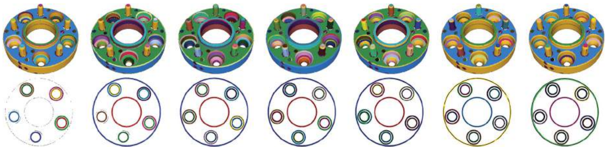
Fig. 14. Effect of various values of the slice's thickness \tau . Leftmost: too fine slicing makes the projection image too sparse for circle detection; Rightmost: too coarse slicing makes the profile curve too sparse for circular primitive detection. (For interpretation of the references to color in this figure, the reader is referred to the web version of this article.)
