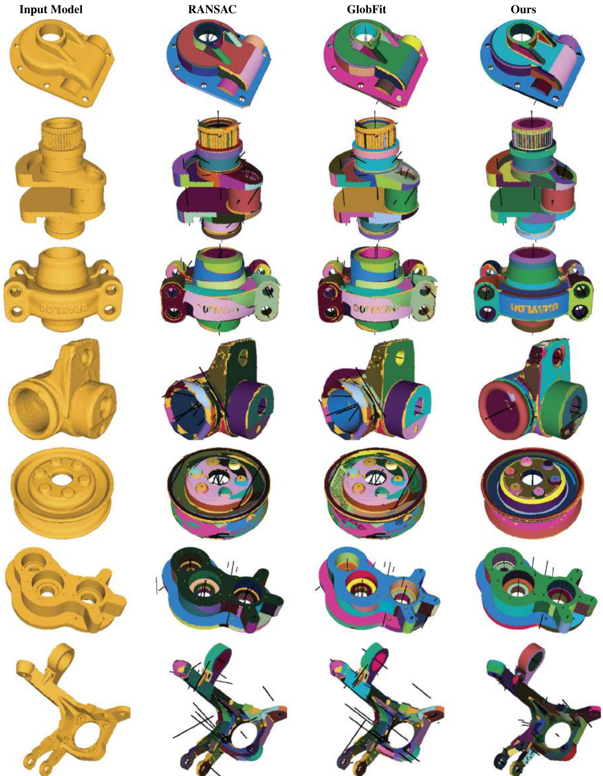
Fig. 1. Failure case of RANSAC-based approach (Schnabel et al., 2007) and GlobFit (Li et al., 2011). First column: Input model (point cloud); Second column: Segmentation from RANSAC-based approach is locally optimal (black lines indicate the axes of the primitives); Third column: GlobFit's optimization can align the parallel primitives but increase the fitting error and fail to recover the correct segmentation; Last column: Our segmentation. (For interpretation of the references to color in this figure, the reader is referred to the web version of this article.)
